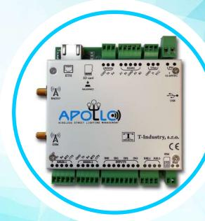
RTU Apollo is based on a powerful 32-bit ARM 9 processor family. It enables communication via Ethernet, integrated  $2G/4G/5G^*$  modem respectively. A webserver is implemented inside the unit, allowing direct user interaction. Communication with the cloud is provided by http REST Api.
