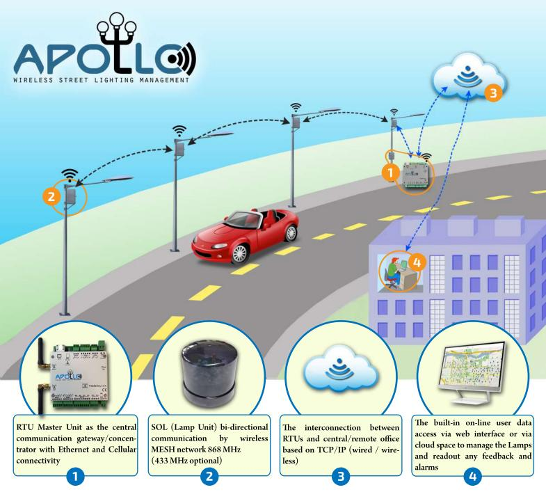
**Apollo (Smart Street Lighting System)** is a comprehensive solution that provides on-line, duplex wireless communication with particular street lamps. It allows sending commands for setting the light intensity, provides feedback signals watching the street lamp state (temperature, power consumption ...) and potential failures (overheating, etc.). It provides a built-in user data access via web interface or via cloud space.
